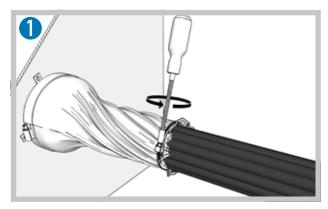
Remove or loose the cable tie holding the cables.
