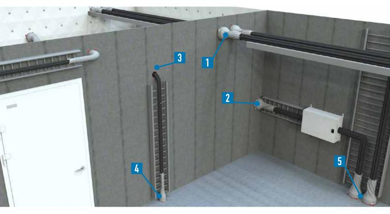
Generally, Easy Transit has a cable filling degree of 0-100%, which means it can be filled visually full. The installation can be done on both sides of the bulkhead, making the installation easy and accessible.
