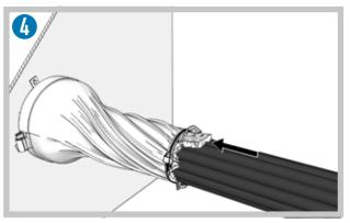
Fill any gaps between cables and/or cable and the wrap with enclosed Marine Blanket. The spare Marine Blanket is placed inside the wrap.
