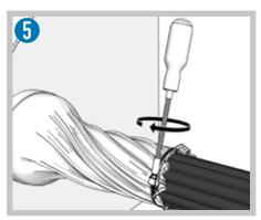
Secure the fireproof wrap with the supplied cable tie. Use a Hex 7mm/Ph2 screwdriver.
