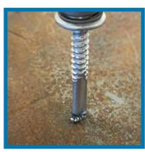
The supplied self-drilling/tapping screw can be used up to 12mm / 1/2 inch thick steel plate. For best drilling results a tight 8mm Hex socket should be used. The screw must not wobble as it reduces the drilling performance. Attention, max 1500rpm, as well as a high working pressure on the screwdriver is recommended.
