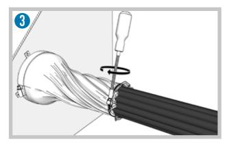
Secure the cable tie over the cables.
