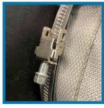
The metal cable tie has a practical quick release function that makes it easy to preload by hand and then tighten with a screwdriver. It is possible to use both a Hex 8mm socket, or a Ph2 screw bit. The cable tie can be easily released and re-installed for retrofit installations.
