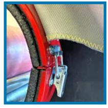
When taping the wrap to the graphite collar, it is easiest to start taping just to the left of the graphite collar's metal lock. By doing so you avoid getting the metal lock in the way of the metal cable tie's lock when it is to be tightened later.
