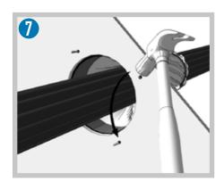
To avoid cut hazard, it is optional to remove the drilling tip by using pliers, hammer or a pipe with an inner diameter of Ø6mm.
