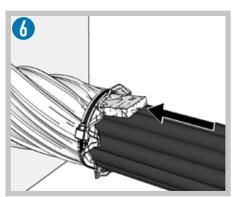
Fill any gaps between cables and/or cable and the wrap with enclosed Marine Blanket. The spare Marine Blanket is placed inside the wrap.
