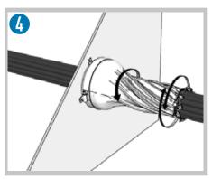
Twist the end of the fireproof wrap counterclockwise to create a smoketight penetration.
