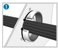
Place the graphite collar over the cables and lock it.
