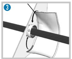
Take the openable wrap, remove the film from the tape and place it on the collar. Secure the wrap with the supplied cabel tie.
