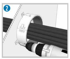
Fasten the graphite collar to the bulkhead or deck with the enclosed self-taping screws. To be installed on one side only.
