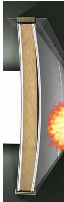
Most of the flexural strength of the panel is lost when the bond between exposed face and core fails. Panel dead load is then carried by suspension cleats.
