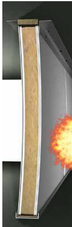
Panel bows towards fire; the floor will still carry the dead load of the panel.
