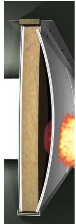
The cold side of the panel bows outwards away from fire when temperature rises and the external steel sheet expands. Panel dead load suspended by cleats.
