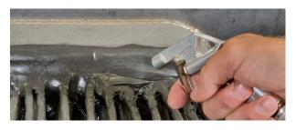
Use compressed air with a nozzle inside diameter of 12 mm (0.5 in.). Air pressure shall be at least 2 bar (2 kgf/cm2, 30 psi) and be at a perpendicular distance from the seal not exceeding 400 mm (16 in).
