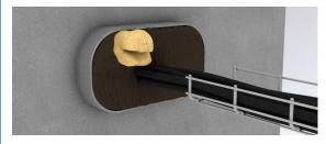
Smooth out the surface of the Marine Flex Sealant using a sponge with soapy water or a piece of Marine Blanket.
