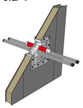
Marine Blanket is cut into suitable stripes. The width of the Marien Blanket stripes should be 24 mm less than the wall thickness.
