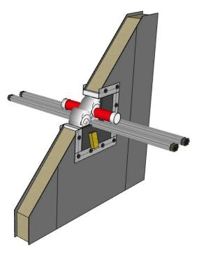
Smooth out the Marine Flex Sealant surface with a scraper.
