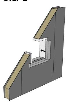
Cut the L-profile to fit the cut-out. Place the L-profile of stainless-steel min. 40x40x1,5 mm, on each side of the sandwich panel opening.
