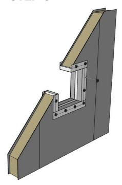
The L-profile is fixed with selfdrilling screws 5,5x135 from one side so the L-profile is secured from both sides.
