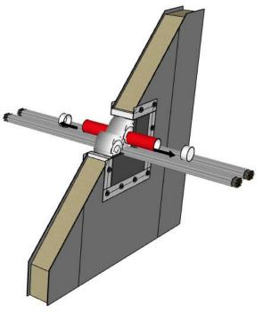
Remove the lids on the **Intumescent sleeve** (red tube).
