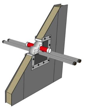
When the Marine Blanket is installed in the wall transit, it's time to start applying the Marine Flex Sealant.
