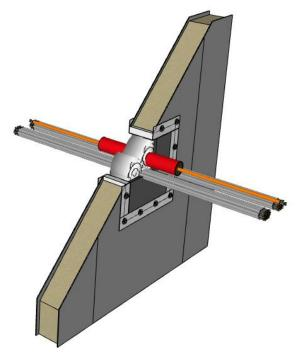
Seal one side of the **Intumescent sleeve** with Marien Flex (min. 7 mm thick) for a gastight installation.
